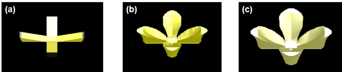
Fig. S10 The perspective view of the Ag-Pt catalyst structures used in FDTD electromagnetic simulations: (a) structure #1, (b) structure #2 and (c) structure #3. The heights of the structures are 200 nm, 500 nm, and 570 nm, respectively.
